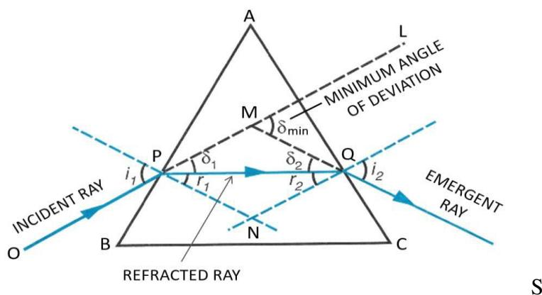
The light from P bends towards the normal. In the glass prism, the ray of light moves along PQ. At the point Q on the other refracting side AC of the prism, the light ray meets a boundary between glass and air.
