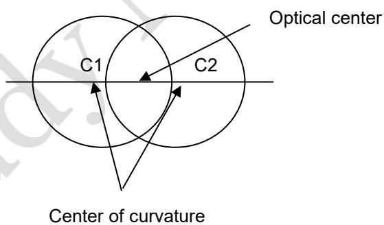
The center of curvature of a lens is the center of the sphere of which the lens is a part. A lens has two centers of curvatures.
